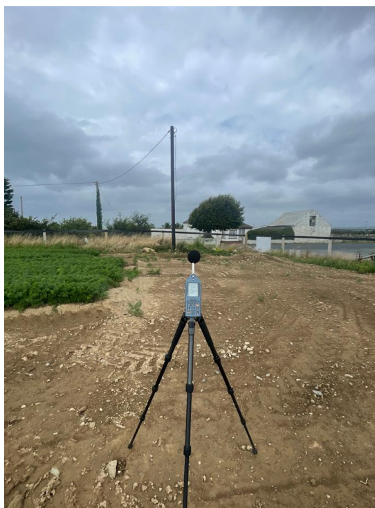
Figure 9-3: Attended measurement setup.
